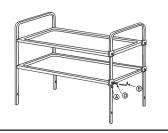
So Insert Casters (B) into the side frames from the bottom. Align holes in caster, side frame and shelf then use screw and nut to connect. Thighten screws to fix the bottom shelf and the casters.
